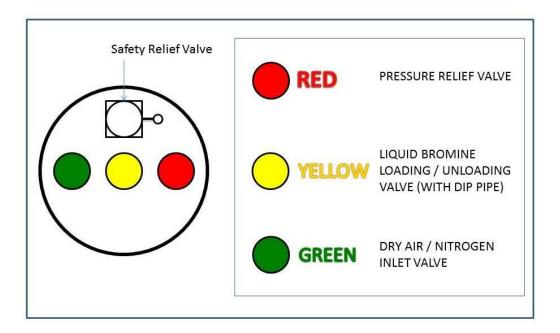
The schematic shows a typical tank truck's unloading set-up. We recommend Teflon lined rubber hoses for the unloading of the trucks.
